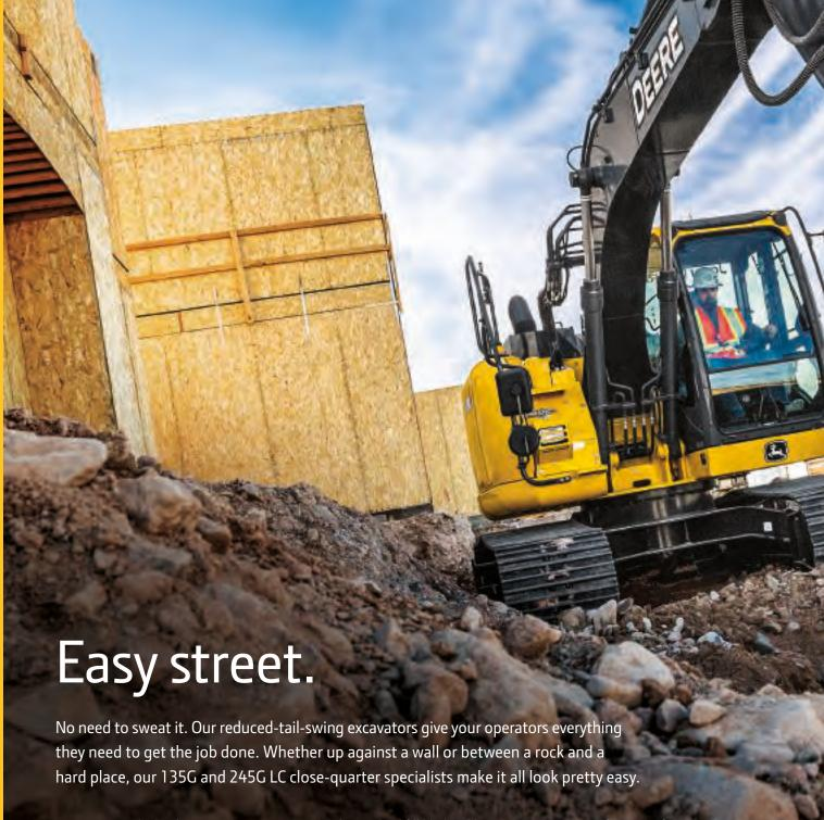
Powerwise™ III hydraulic management system perfectly balances engine performance and hydraulic flow for predictable operation. Three productivity modes let an operator choose the digging style that fits the job. *High-productivity* delivers more power and faster hydraulic response to move more material. *Power* delivers a balance of power, speed, and fuel economy for normal operation. *Economy* reduces top speed and helps save fuel.
