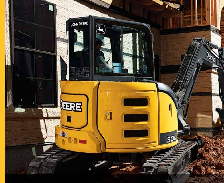
Power/economy work modes allow you to match engine speed to the application. Select **Power** mode and get the higher engine speeds needed for most general digging work. For lighter digging demands, **Economy** mode reduces engine speed and noise, while improving fuel efficiency.
